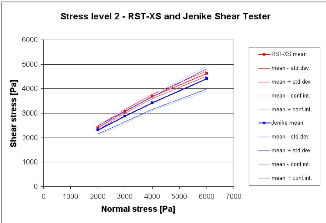
Abb. 5.9: Mean shear stress  $\tau_m$  (mean), range of standard deviation  $\tau_m \pm s$  (mean  $\pm$  std.dev.) and 95% confidence interval  $\tau_m \pm a$  (mean  $\pm$  conf.int.) of Jenike shear tester [2] (blue), ring shear tester RST-XS (red). Values have been measured at stress level 2.
